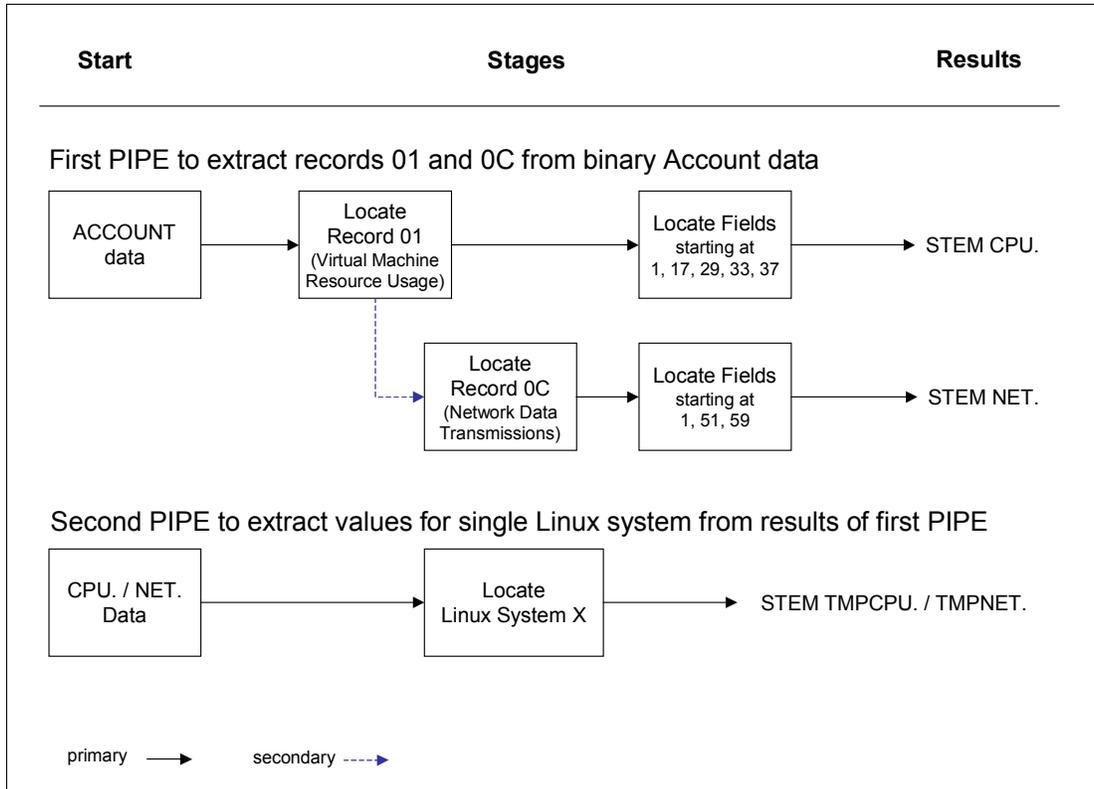
Figure 2 Extraction pipe flow
