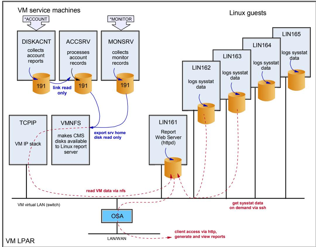
Figure 1 System configuration
